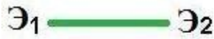
Fig 7. Function model. E1 is a subject of function (tool), while E2 is an object of function (product).
